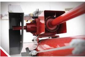
**GEAR BOX** Heavier gear boxes feature oil baths, forged steel gears and quality roller bearings.
