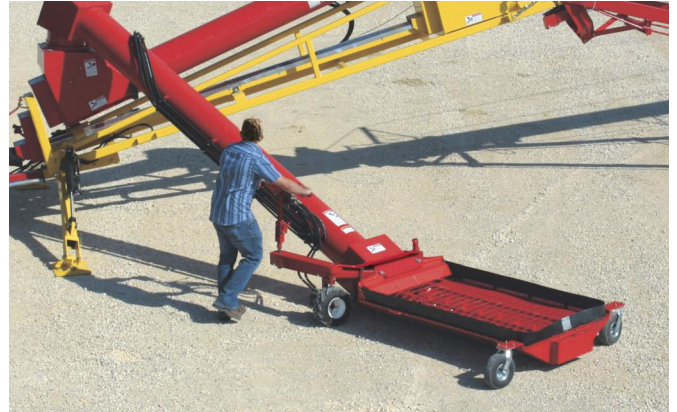
Hydraulic Drive Positions the Hopper with Ease
