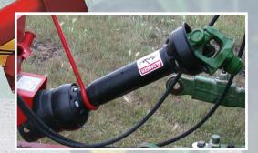
**CV-PTO Shaft** All MK augers are equipped with an overload shear bolt. The CV-PTO shaft, assures smooth operation with vibrationfree running, longer wear and constant
