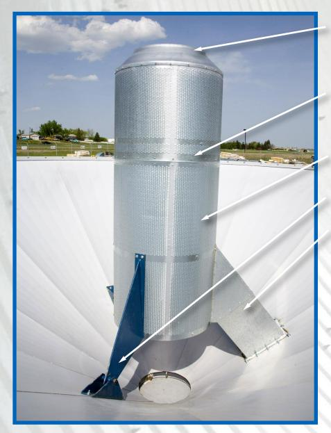
The 20" Inside Diameter and Perforated Core forces air up into the center of bin to allow uniform drying and reduced unloading bin pressure.
